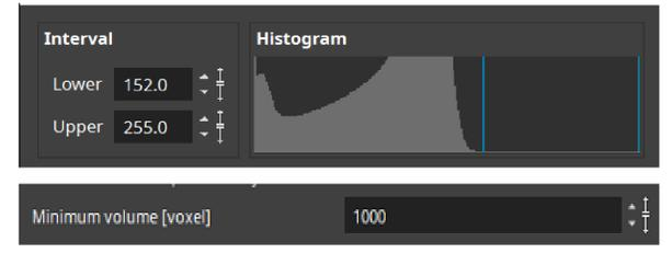
Grey-scale thresholding was employed for segmentation (demarcation of 3D regions of interest) and a minimum voxel size of 1000 voxels was maintained for all the samples to establish consistency.
